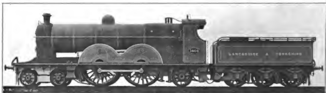
Fig. 5057. Ten-Wheel, Four-Coupled Locomotive. Lancashire & Yorkshire. Cylinders 19 in. x 26 in.; Working Steam Pressure 180 lbs. per sq. in.; Total Heating Surface 2,052.6 sq. ft.; Diameter of Drivers 87 in.; Weight on Drivers 78,400 lbs.; Total Weight 131,600 lbs.
